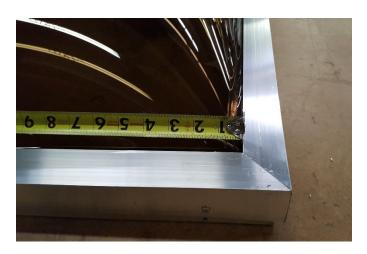
AND THAT'S IT! From this, we can deduct about 1/2" from the outside dimensions to get the tip to tip/overall dimensions on the dome, and we will generally match the inside dimensions to the rise to rise dimension on the dome. Flange dimension is resultant of overall less rise to rise divided in half. 20-25% rise is standard. Thickness is dictated based on part size.
