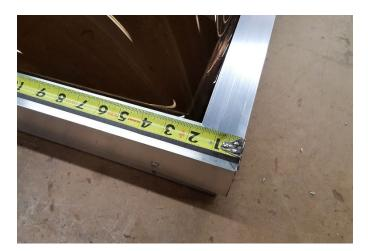
WHAT TO MEASURE: "DAYLIGHT OPENING"/INSIDE RETAINER: \_\_\_\_\_\_ (width) x \_\_\_\_\_\_ (length)
